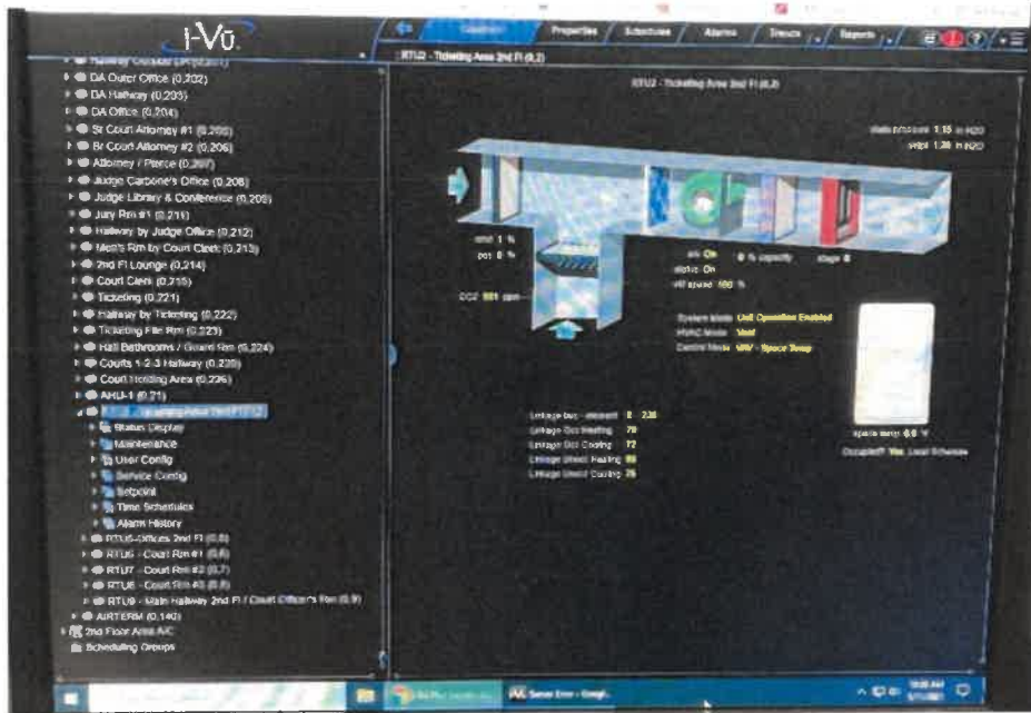
Figure 16: Typical RTU BMS Screenshot
