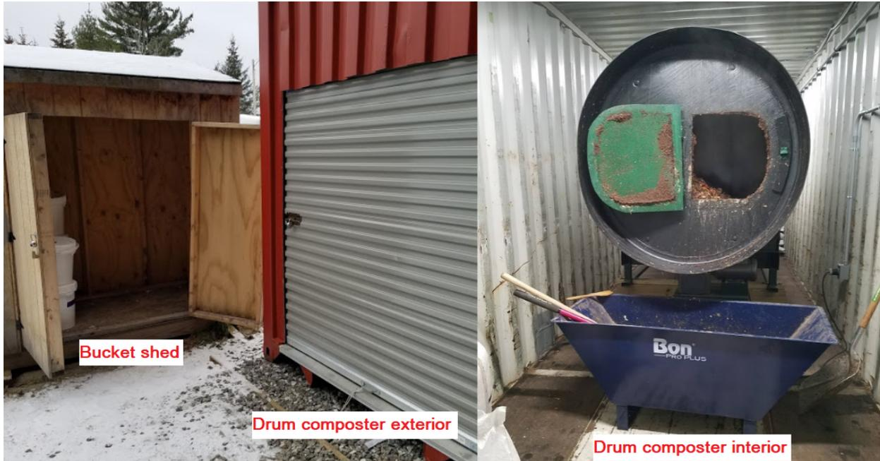
Photo 2: Components of the drum composter system
