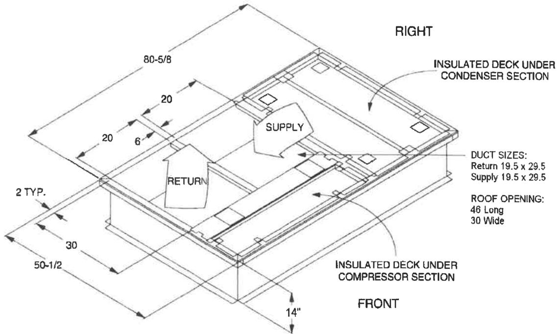
\* Supply and Return Air (Including duct support rails) as shown, are typical for bottom duct applications.
