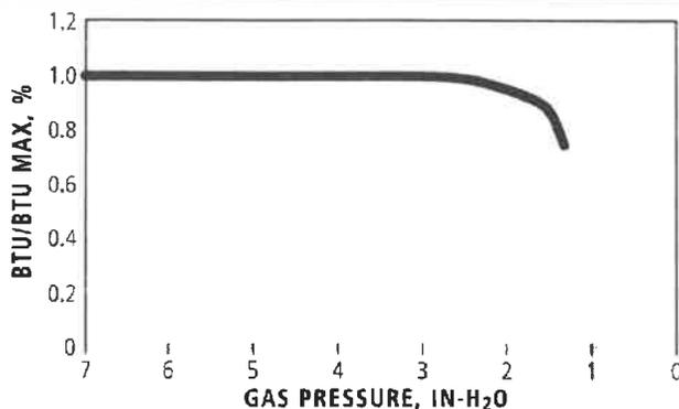
FlexCore units are capable of full-fire output at a minimum of 3" wc.
