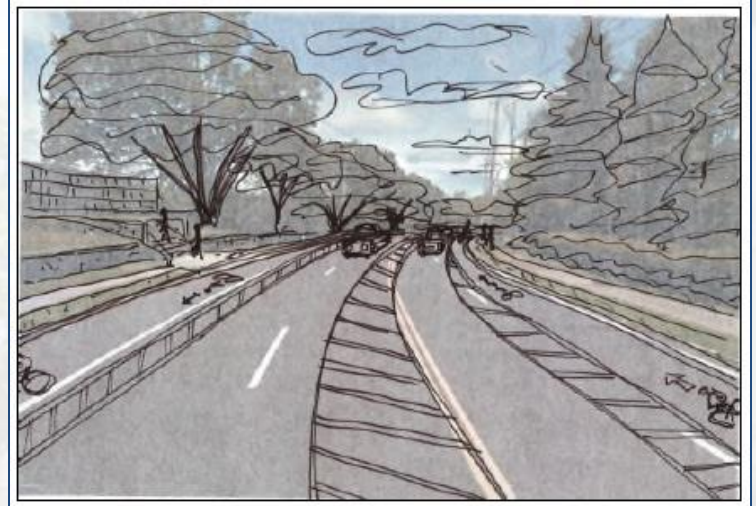
Striped Median and Bicycle Lane Buffers
