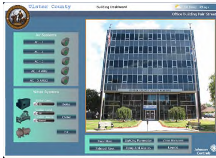
Figure 4: Johnson Controls Metasys Building Automation System
