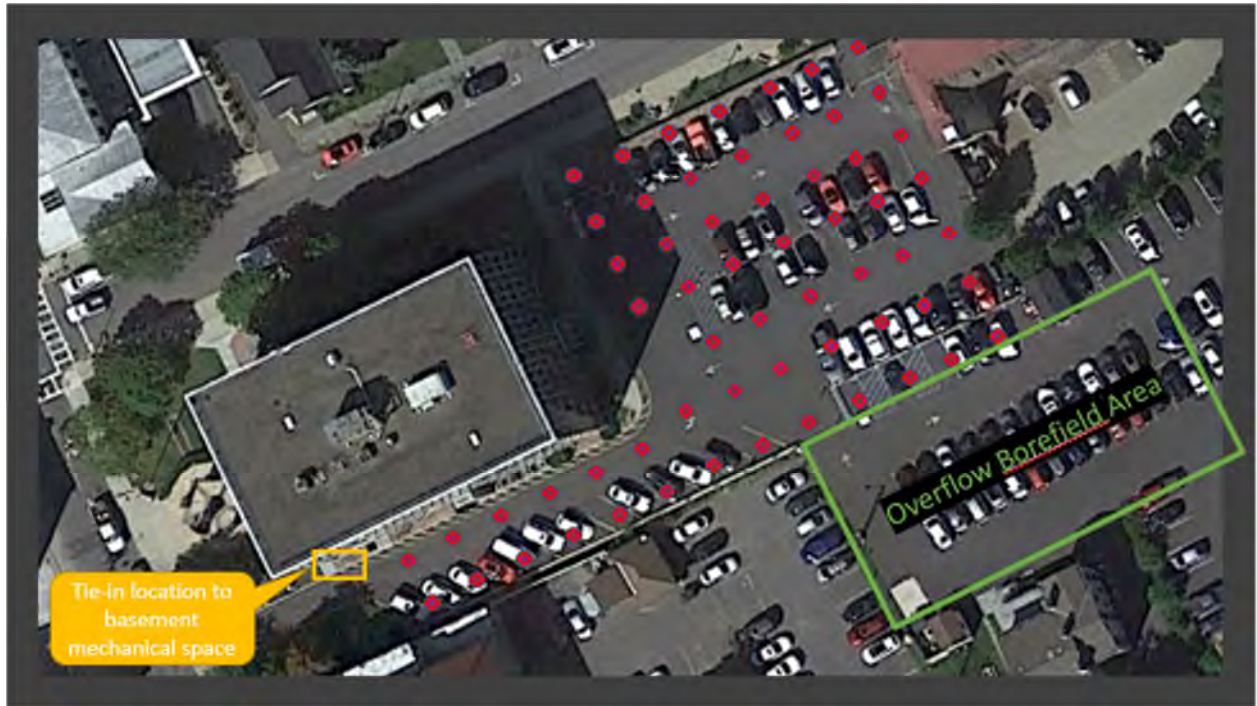
Figure 18: Heat Exchanger grid layout
