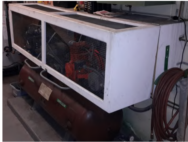
Figure 5: 1.5 HP DeVilbiss air compressor
