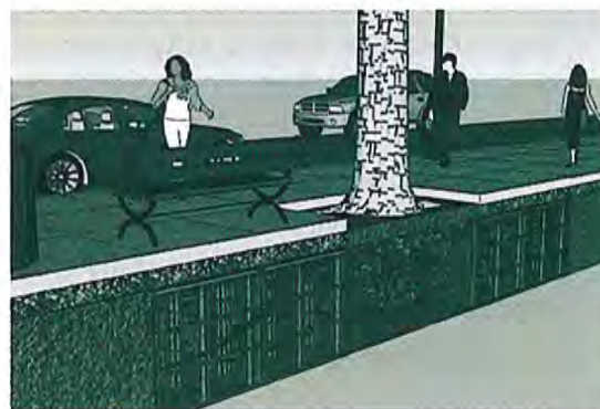
Figure 17 Silva Cells below permeable paving Copyright 2008. Casey Trees. Washington D.C.
