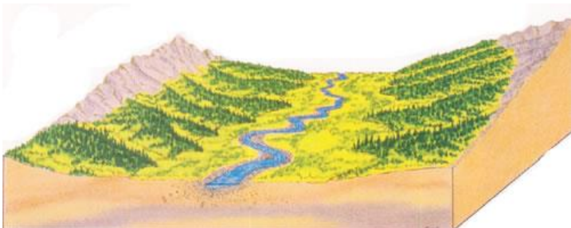
Figure 4: Rendering of the Rosgen “C” stream type.
