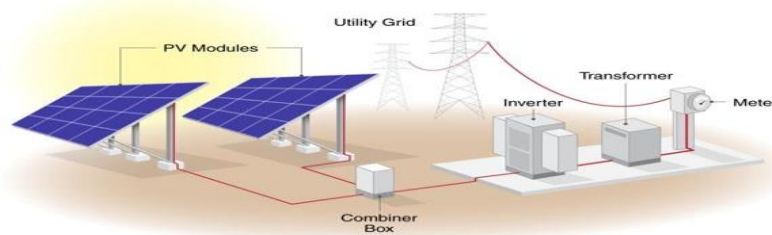
Figure 6. Ground mount array (source: NREL)
