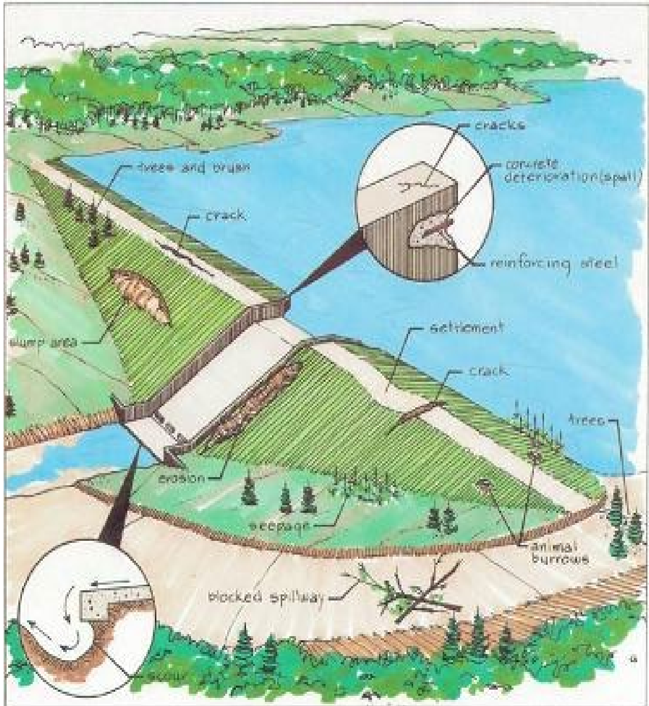
Signs of deterioration in dams. Source: British Columbia Dam Safety Guidelines.
