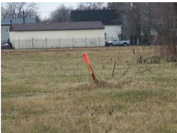
Monitoring well on site
