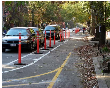
Flexible bollards can delineate a path along the Elementary School driveway
