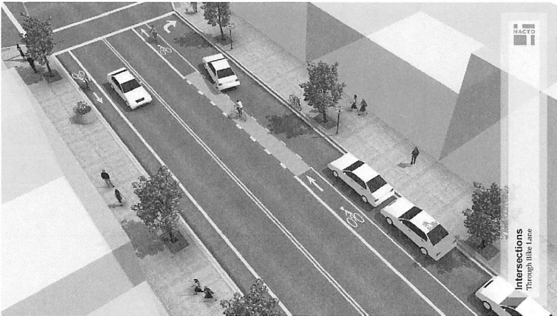
Figure 52 Example of a Painted Merging Area Between a Bike Lane and Right Turns for Vehicles
