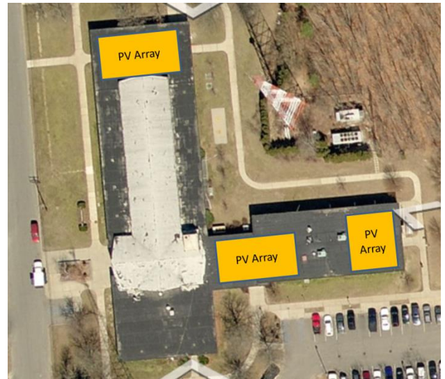
Figure 32: Roof of Probation with possible PV array arrangement.
