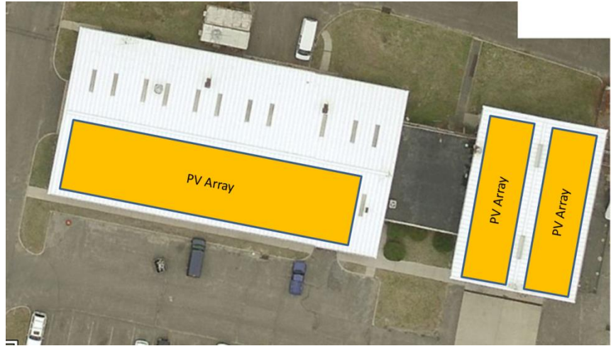
Figure 30: Roof of Custodial Warehouse with possible PV array arrangement.
