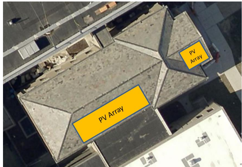
Figure 35: Roof of Supreme Court Building with possible PV array arrangement.
