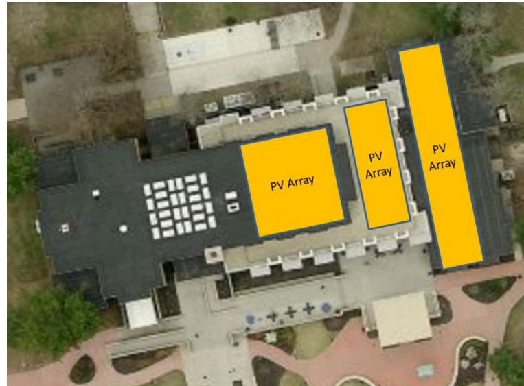
Figure 7: Roof of Ammerman Building with possible PV array arrangement.
