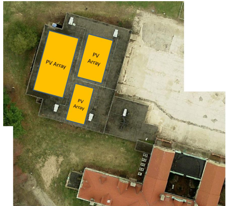
Figure 8: Roof of Coindre Hall with possible PV array arrangement.
