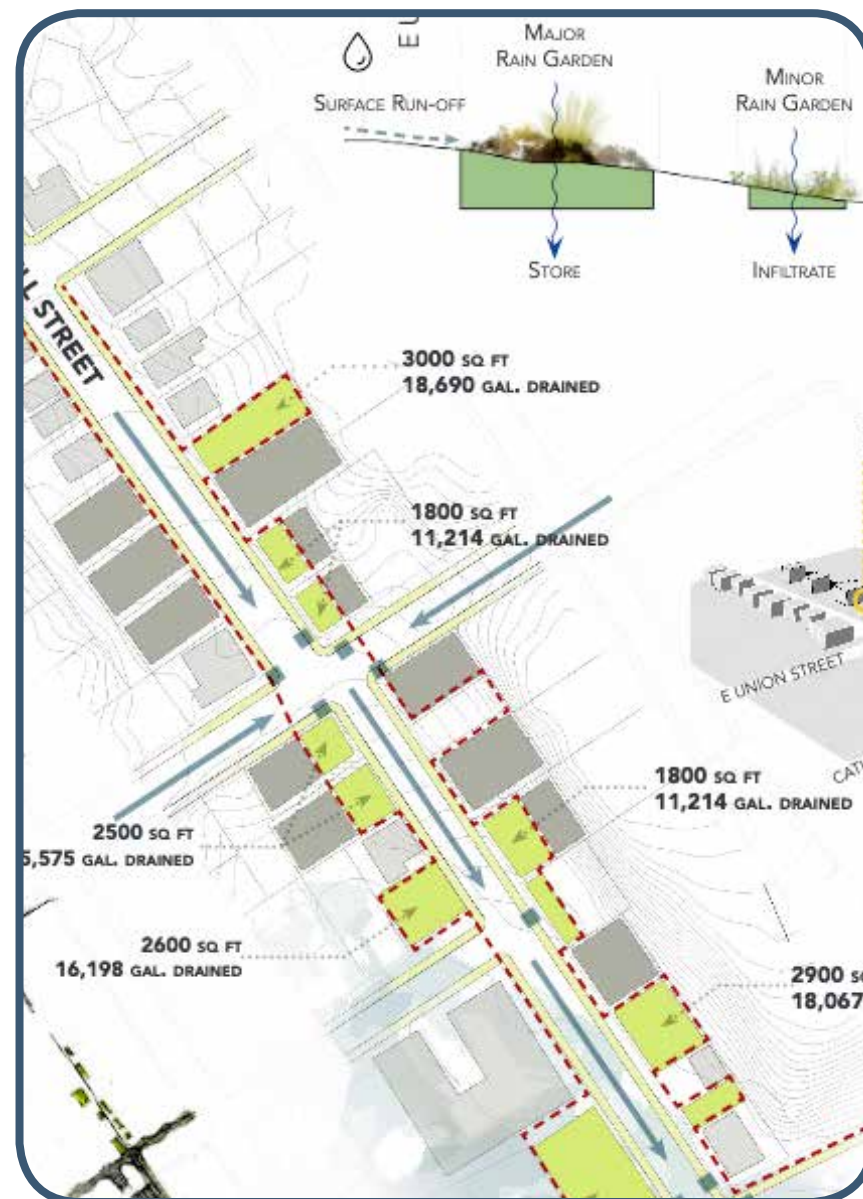
A stormwater planning concept illustrating possible locations of rain gardens that could be installed over time
