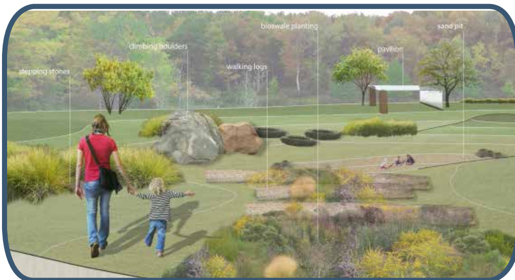
A vegetated swale designed to capture stormwater running through a city park
