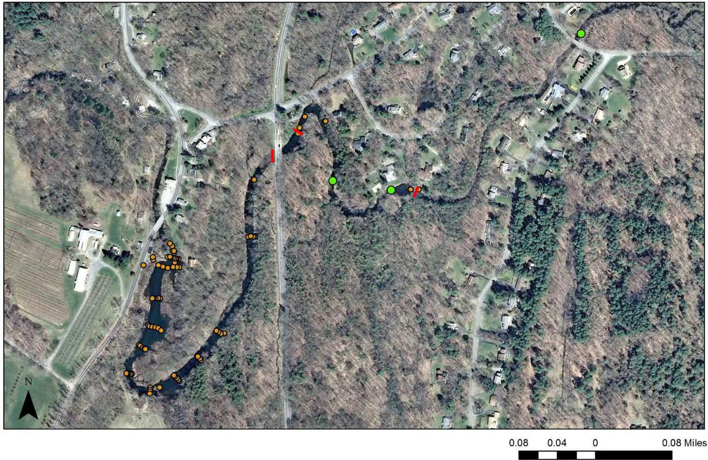
**Figure 5.** Map of bathymetric and depth of refusal survey data collected at Annandale Dam (orange points) and other inspection points (green). Locations of observed bedrock seams are shown as red lines. The furthest upstream bedrock seam shown on the map corresponds with the upstream extent of the impounded water surface during low-flow conditions.
