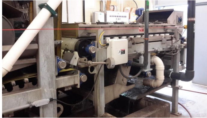
Figure 8: Belt filter press in the Main Building
