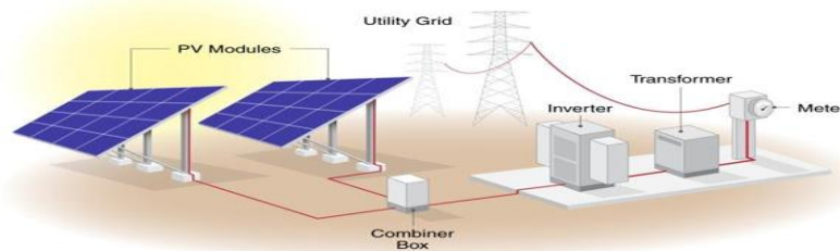
Figure 6. Ground mounted array (source: NREL)
