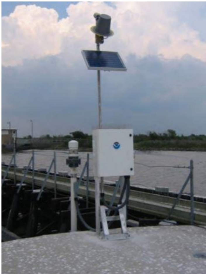
Figure 12. A NOAA telemetry station as depicted in the USGS handbook, (Sauer, 2010).
