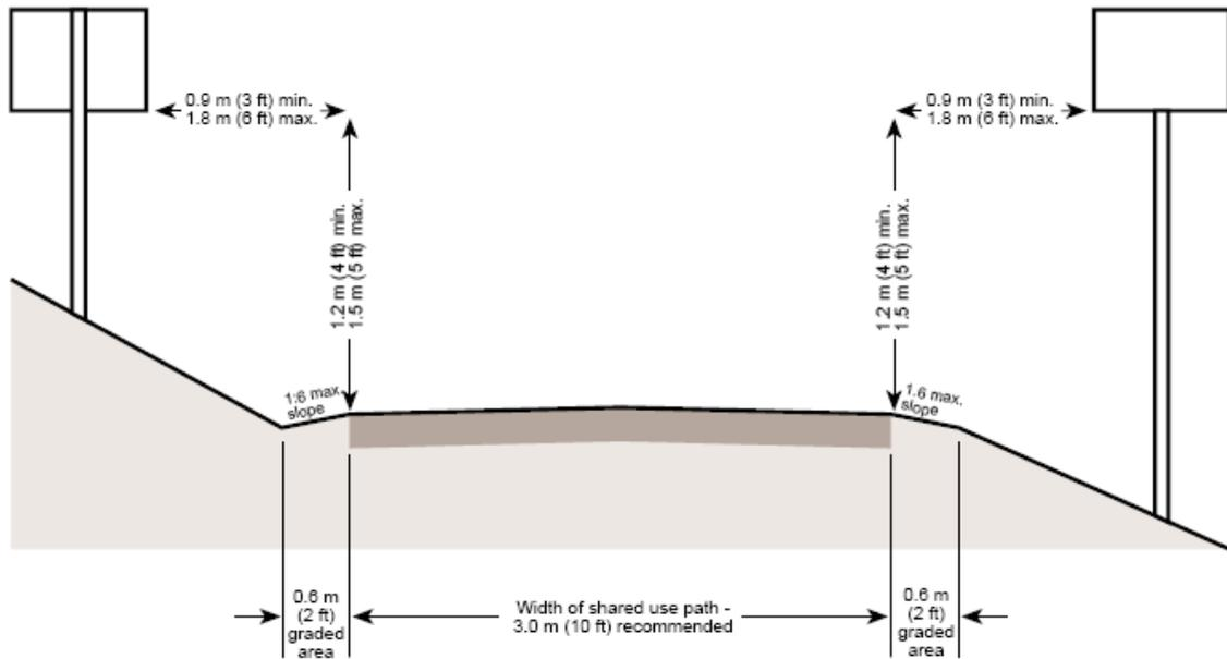
Shared-use path cross-section from the *AASHTO Guide for the Development of Bicycle Facilities*. This is the most commonly used trail facility guideline in the U.S. Projects built to this cross-section are eligible for most federal and state transportation funding sources.
