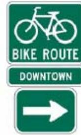
The *Manual of Uniform Traffic Control Devices* provides specific design details for the placement, and size of standard bicycle facility signage. All bicycle facilities within Ulster County should be signed per the MUTCD. In general, the sizes of signs used on bicycle paths are smaller than those used on roadways. If the sign applies to drivers and bicyclists, then the larger size used for conventional roads should apply.
